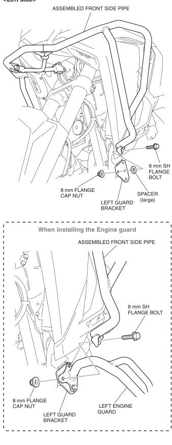
26. Raise and install the assembled front side pipe center stay as shown.
