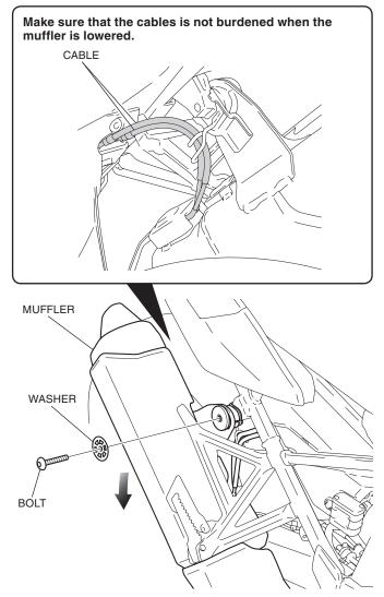
13. Remove the parts as shown. **<Left side>**
