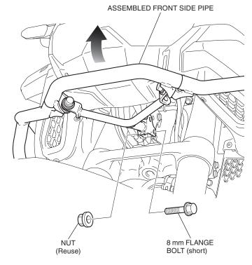
27. Install the parts as shown.
