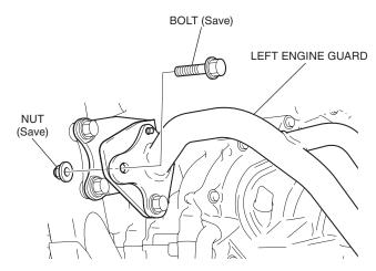
25. Loosely install the assembled front side pipe as shown.
