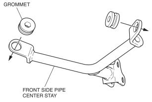
21. Install the collars to the front side pipe center stay as shown.
